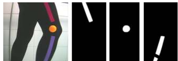
Fig.5. Thresholded image processing through morphologic techniques.
